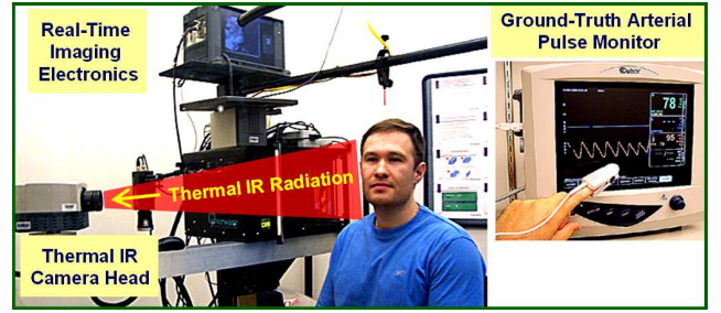
Figure 7. Experimental setup. The thermal sensor used in the experiments for this paper is a long-wave Phoenix IR camera from FLIR [1]. Multi-parameter contact vital signs monitor "Advisor" was used for ground-truth measurements [2].
